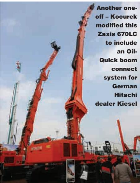
**Another one-off - Kocurek modified this Zaxis 670LC to include an Oil-Quick boom connect system for German Hitachi dealer Kiesel**
