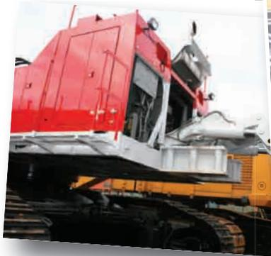
**The counterweight will be hydraulically attached and removed as required. It had yet to be fitted at the time of D&Ri's visit**
